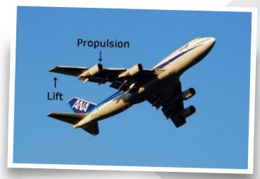
The binary actions to make an airplane fly begin by producing the propulsion that generates the necessary speed of the airflow on the wings of the airplane to generate the lift.
