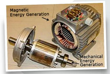
The binary actions of the process are, on the one hand, the transformation of electrical energy into magnetic energy and, on the other hand, the transformation of the magnetic force into mechanical energy. These processes happen within the rotor and the stator of an electric motor.
